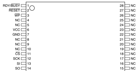
Figure 2-2. CASON – Top View through Package
