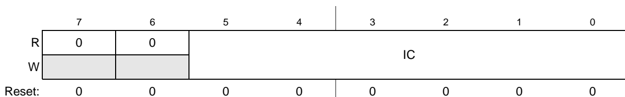
Figure 24-3. I 2 C Frequency Divider Register (I2FDR)
